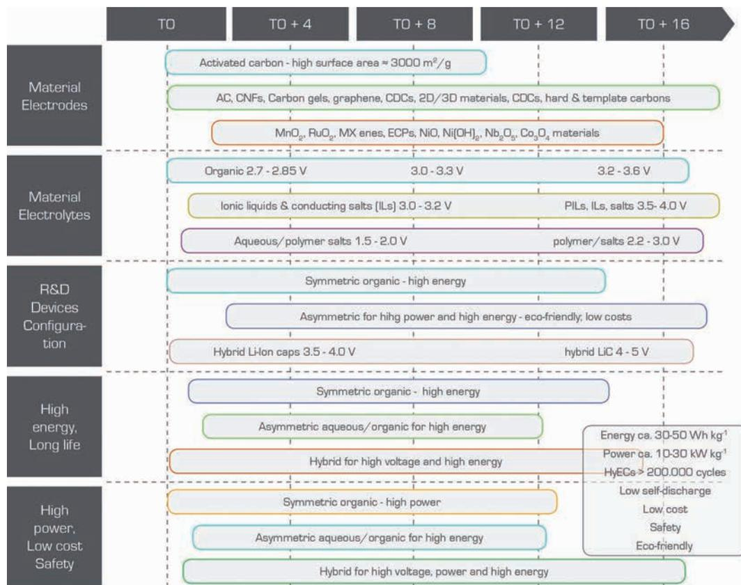
Figure 9: Tentative Roadmap for supercapacitors with vision to 2030. Prepared by CNR-ITAE based on several sources<sup>80</sup>.
