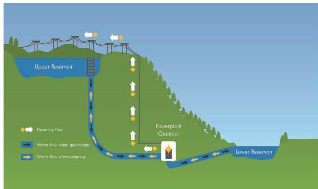
Figure 14: Principle of a Pumped Hydro Storage plant. Source: New Civil Engineer, 2016.
