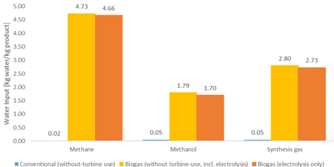
**Figure A3.2.** From cradle to gate water input for production of basic chemicals and polymers from carbon capture and utilisation process with biogas as CO<sub>2</sub> source. The water input for electrolysis is actually consumed water that is chemically transformed in the process. The electrolysis causes an increased water demand, as water is used as a raw material, which is not the case in the conventional route.<sup>58</sup>
