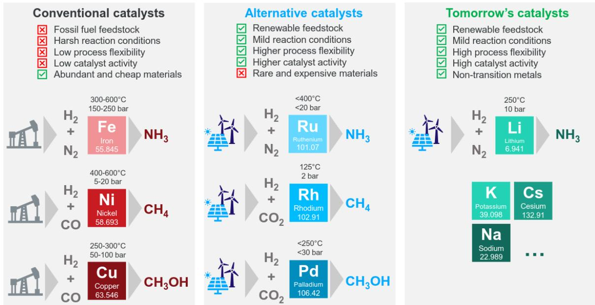
**Figure 19.** Quest for earth abundant catalysts. With its short-to-long term perspective, SUNERGY works on solutions for the three classes of catalyst materials - from conventional, to alternative up to tomorrow's catalyst. Source: [ENGIE Emerging Sustainable Technologies: collaborate to reach carbon neutrality report](#).
