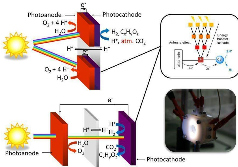
**Figure 10.** SUNERGY's R&I Focus Area of direct solar conversion via integrated artificial photosynthetic systems. SUNERGY addresses the conversion of CO<sub>2</sub> into a variety of products, the transformation of atmospheric nitrogen with green hydrogen to produce ammonia for fertilisers and, more generally, the direct solar-powered production of fuels and chemicals. Graphics: courtesy of SolHyCat.
