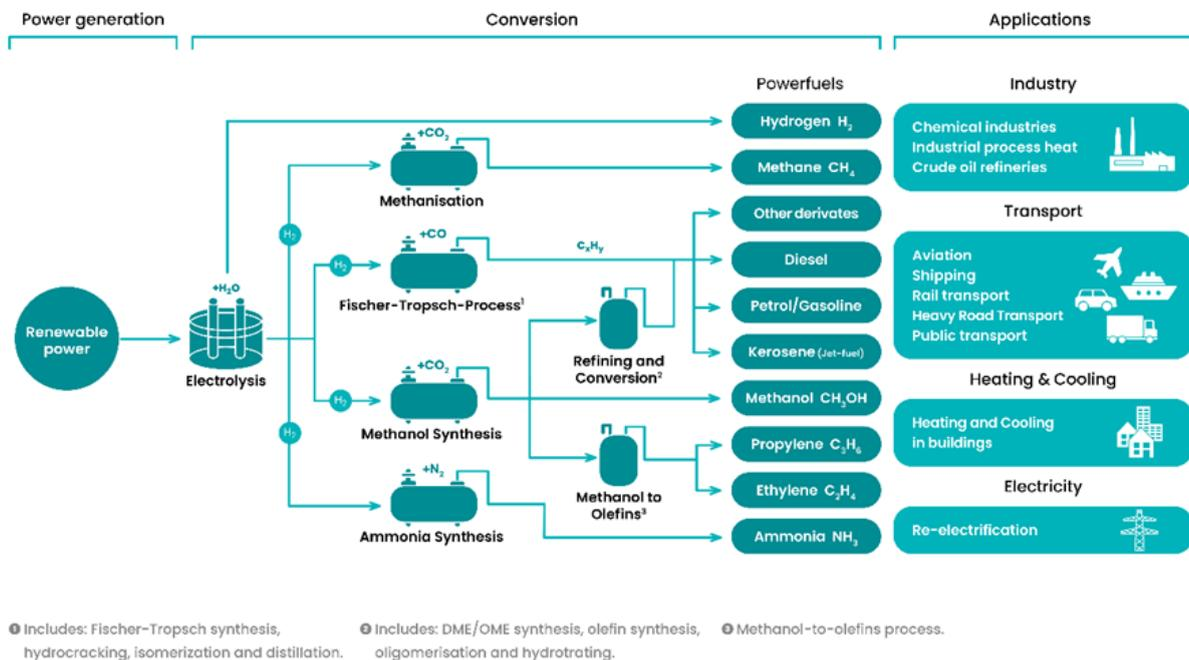
**Figure 6.** Illustration of a sustainable energy system based on multi-step renewable power conversion. Several components are industrially well-developed at present. E-fuels are produced from renewable power, driving the splitting of water into hydrogen and oxygen. In subsequent conversion
