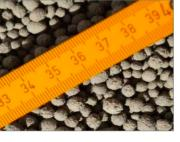
Waste heat recovery and transport Packed bed sensible TES up to 1300°C : **Kraftblock Possibility of direct heat transfer to particle beds**
