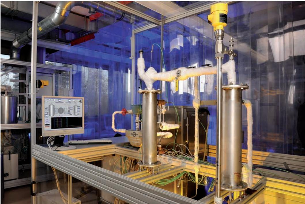
Figure 18: Test stand for thermal upgrade of waste heat at  $T > 140^{\circ}\text{C}$ . Source: DLR.
