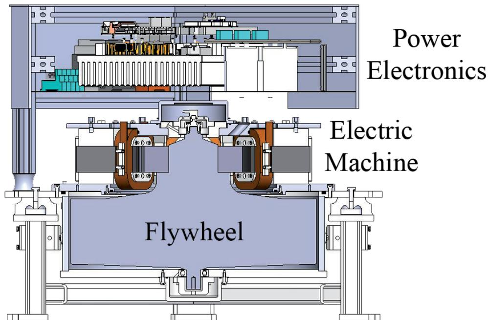
Figure 13: Basic scheme of a Flywheel. Source: CIEMAT.
