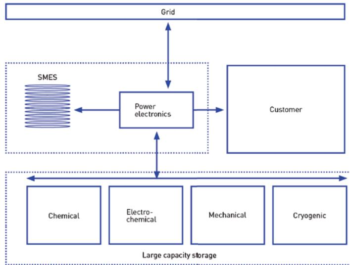
Figure 10: SMES buffering of mechanical, chemical, electrochemical or cryogenic Energy Storage Systems.
