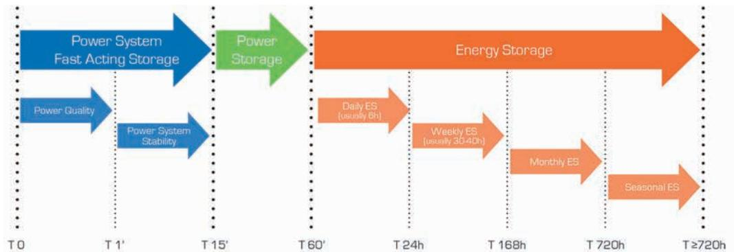
Figure 2: Energy storage applications segmented by discharge time<sup>29</sup>.
