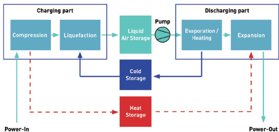
Figure 12: LAES mode of operation.
