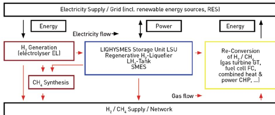
Figure 11: LIQHYSMES Storage Unit based on hydrogen for long term energy storage and SMES for short term storage<sup>86</sup>.
