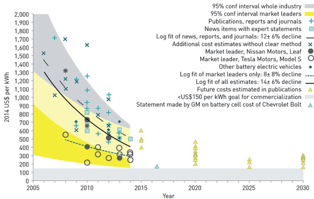
Figure 8: Cost estimates and future projections for electric vehicle battery packs, measured in US \$ per kilowatt hour of capacity. Each mark on the chart represents a documented estimate reviewed by the study. Source: Nykvist et al. (2015)<sup>73</sup>.
