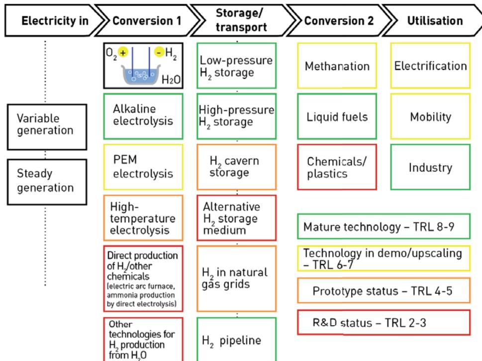
Figure 5: Technical maturity of chemical storage components. Adapted from Siemens, 2012.
